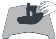
1 Together with the flexible platform after the printed model has been cooled down. Remove from the device
