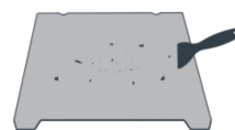
2 The residue of the platform filaments can be scraped off with a blade. Be
