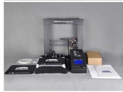
18. Open the Sapre parts box, you will see the USB Cable, Filament Spool Holder, Fiament Spool Stand, 4GB MicroSD Card, Power Cable, a Tool bag(6 Hex Bolts, PTFE Tube, 2 Cable ties and 4 wrenches), a Scraper. and a 0.4mm drill bit.
